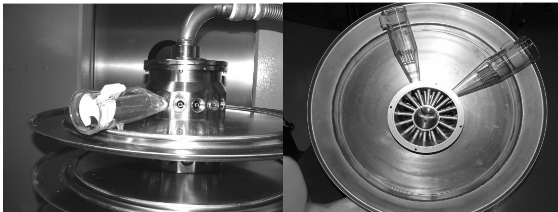
Figure 3: Partial view of the direct-flow nose-only inhalation exposure system (inhalation unit). The picture on the left shows the upper part of the unit with the fume inlet installed, the inhalation ports and, as an example, one acrylic glass tube installed. The picture on the right shows a top view of the inhalation unit with the fume inlet removed, providing a view of the inner inlet cylinder with the stainless steel tubes directed to the inhalation ports as well as the outer cylinder that serves as exhaust drain.
